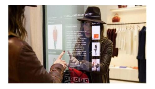
When a customer takes clothing off the hanger, the smart hanger automatically identifies the tag on the taken item, and the information on style, color, price etc. shows up on the display. At the same time, customer's behavior data is uploaded to the server. Through software analysis and statistics, we can get the clothing pick up rate and know which smart hangers attract customers' attention most.
