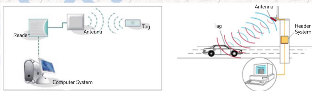
Figure 2.1: The actual application scenario of RFID
