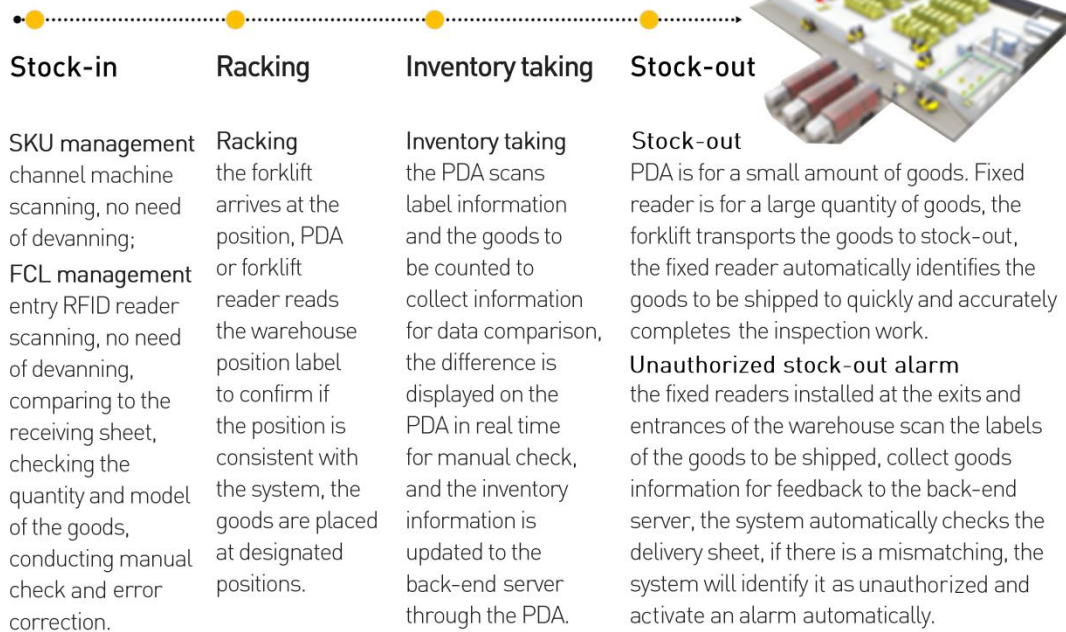
Figure 2.12: The intelligent warehousing solution
