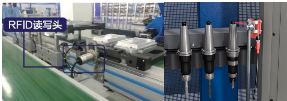
Fig. 3. RFID application on a production workplace
