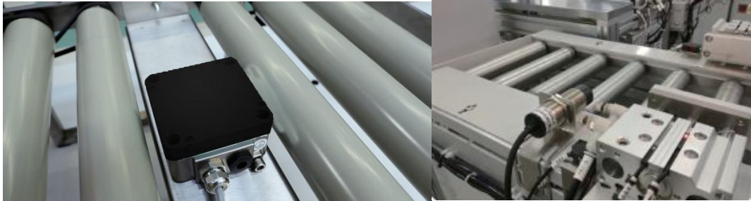
Fig. 4. RFID application on a production conveyer line
