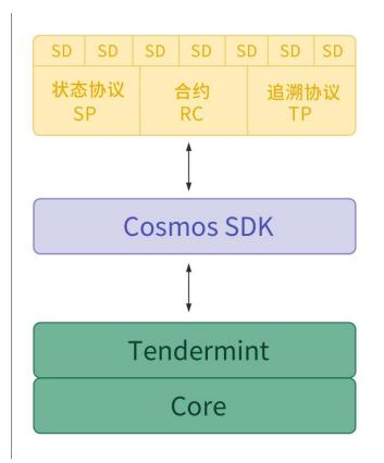
The system architecture of Rainbow Zone consists of a network layer, a consensus layer, and a Rainbow application protocol.
