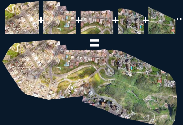
Figure 10: Multiple orthorectified images are stitched together to make an aerial map. [Source: UAS Sky Is The Limit]
