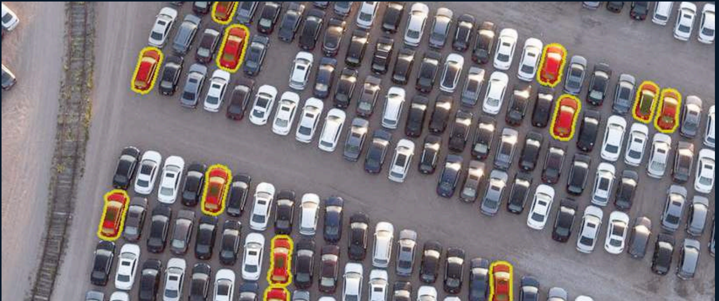
Figure 19: An example of automated object classification for parked cars within a geofenced area. [Source: Takor Group]
