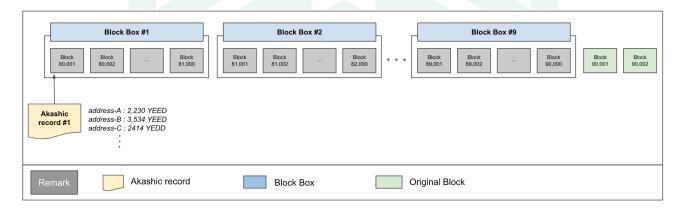
The Akashic Record is a set of data that stores the results of all transactions (the result value of transactions from all accounts) from a Genesis block to a block at a specific checkout point. A Block Box is a set of blocks containing several blocks in one box.
