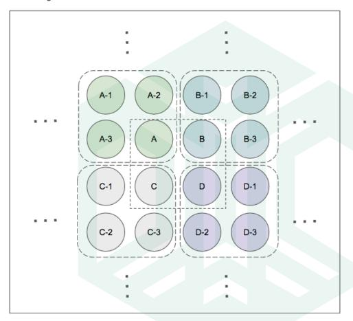
The above diagram depicts the node operating configuration of YGGDRASH. Among the nodes, A-D alphabets are the master nodes, and alphabetic-numeric nodes are sub-nodes of corresponding master nodes. The block generation of the node develops randomly by an algorithm, and the structure has robust tolerance to malfunctions because the empowerment process executes immediately when there is any failure or delay in a certain node.
