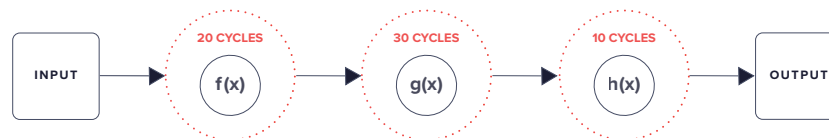
Figure 4: In conventional “Turing-complete” smart contract platforms, an interpreter measures the cost of running a contract, every single time it executes. In Zen, each part of a contract is wrapped in a proven cost. Zen’s contract language uses these costs to verify the cost of the whole contract, before it ever runs.
