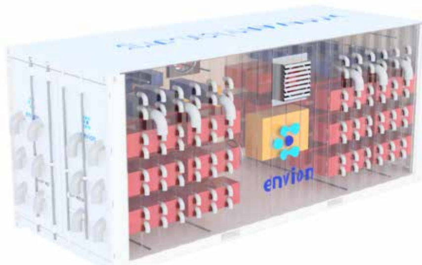
Figure 6. Cooling system & arrangement of hardware. Two large diameter fans decrease pressure inside the container, resulting in directional inflow of cool air through ventilation ducts. Archive racks on rails are used to host the hardware.
