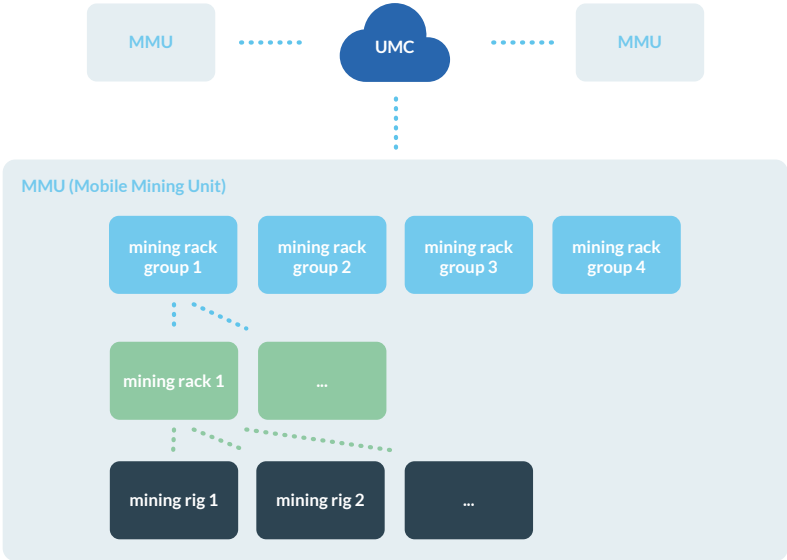
Figure 2. System Overview. Zoom in from Unified Mining Cloud connecting the MMUs to smallest entities. Even at the container's maximum gross weight, our units can be moved and stacked freely by means of simple fork-lift trucks that are capable of lifting 3 tons of weight.
