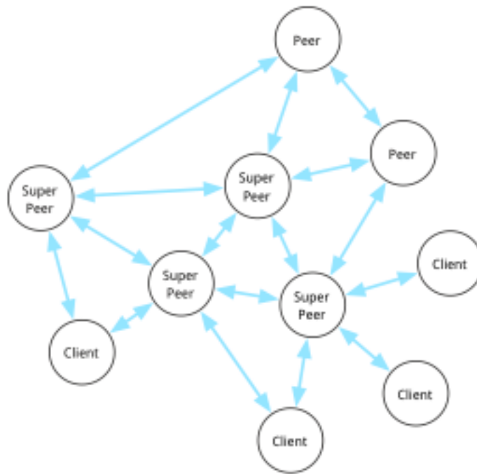
Figure 1. An autonomous 3-tier P2P network.
